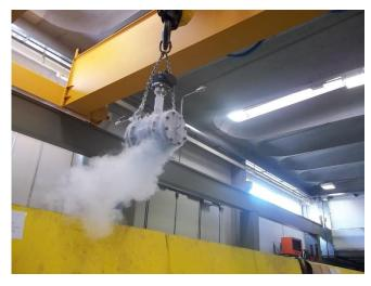
Low Temp. & Cryogenic Test
