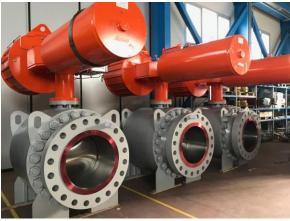
Metal seated with metal sealing and stem extension for steam service and high temperature applications. The special design is suitable for service from 250°C up to 700°C and over
